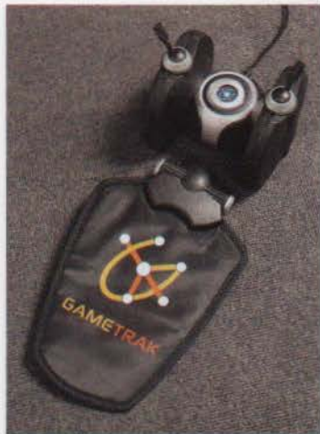
Gametrak's retractable cords will measure depth and direction. The footpad acts as a 'start' button
